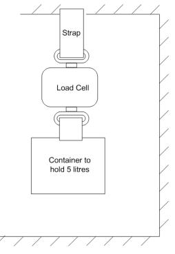
Turn on Telerein and wait for it to complete its start up sequence. The additional weight of the container is "zeroed out" (commonly known as tared), the load cells thus effectively see zero grams force. You may now slowly pour water into the container (weigh it using digital kitchen scales) You should observe the LED colours change at the specified gram force. Put in sufficient water at each step to take you through each of the colour transitions.
