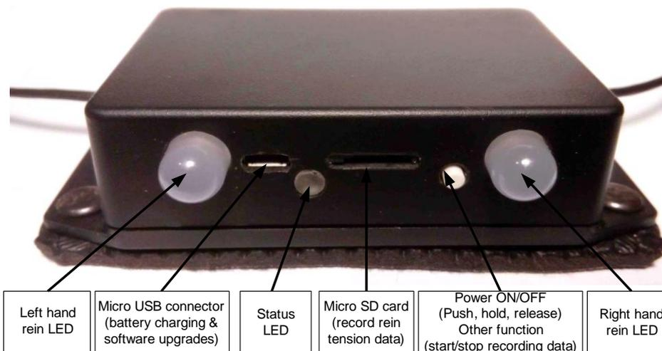
**To turn the unit 'ON'**, gently push down on the white 'Power ON/OFF' button for about 5 seconds until the Left-hand rein and Right-hand rein LEDs start alternately flashing red, then release the button. During this interval, do not touch the reins. Following that, the left and right-hand rein LEDs cycle through the colour spectrum that will be observed in use. Once this cycle completes, the LEDs both display blue, and the unit is ready to use.
